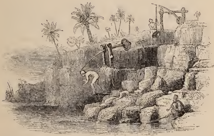
VIGNETTE D. Modern shadóof, or pole and bucket, used for raising water, in Upper and Lower Egypt
